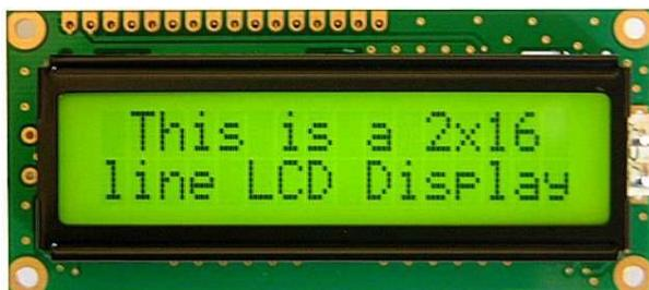
Gambar 4. Liquid Crystal Display (LCD) type 2x16
