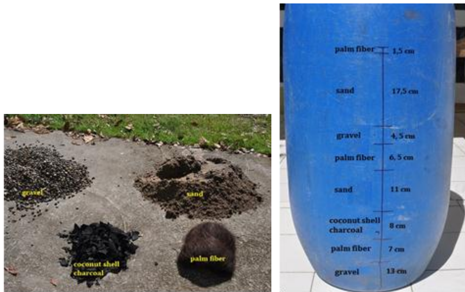
Figure 2. Natural filter and drum with height and thickness measurements
